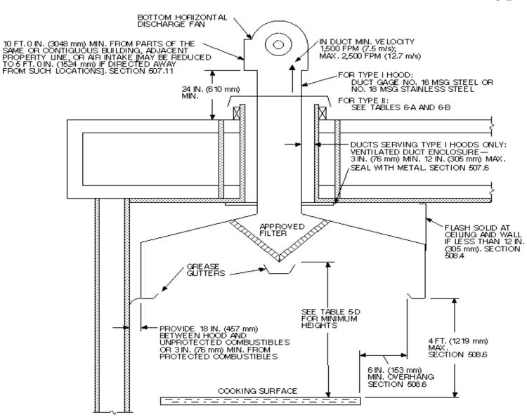
TYPE I HOOD KITCHEN GREASE HOOD GALVANIZED STEEL -- NO 24 MSG STAINLESS STEEL - 0.030 IN. COPPER-24 OZ.PER.FT.
