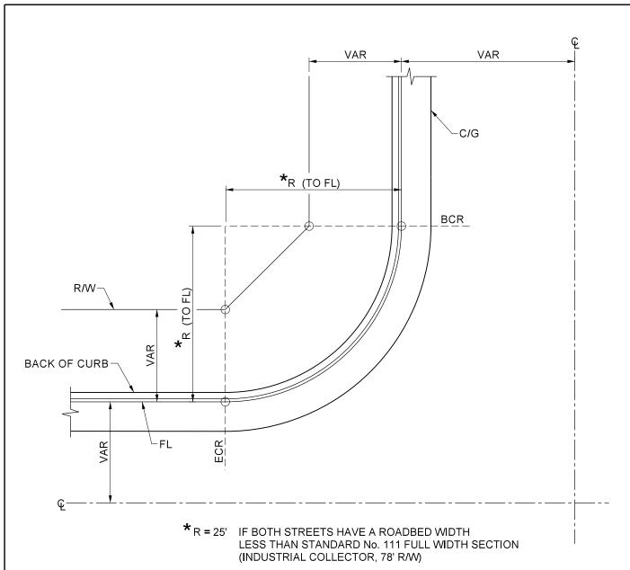
\*R = 35' IF EITHER STREET HAS A ROADBED WIDTH GREATER THAN OR EQUAL TO STANDARD No. 111 FULL WIDTH SECTION (INDUSTRIAL COLLECTOR 78' R/W)
