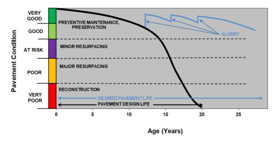
Figure 11. Treatment Zone Alternatives as a Function of Pavement Condition
