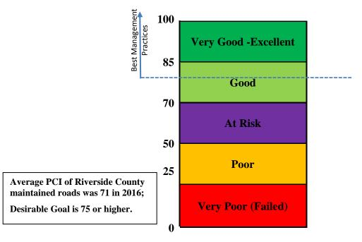
Figure 1. Relationship Between PCI and Condition
