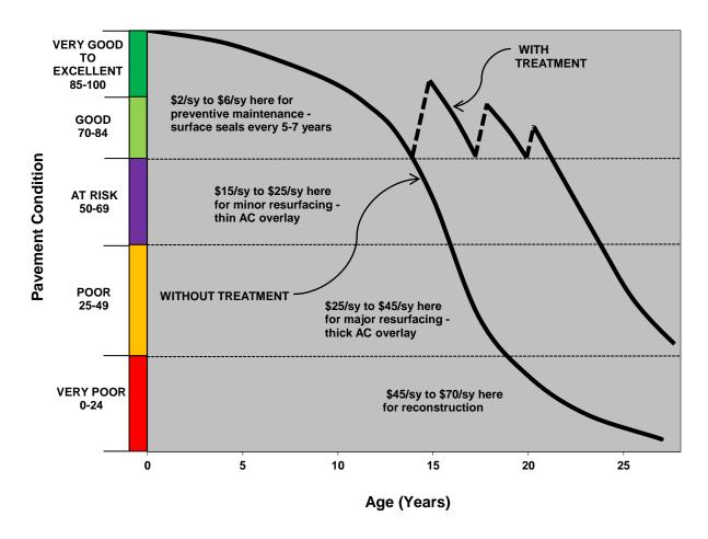
Figure 12. Pavement Deterioration Curve With and Without Treatment
