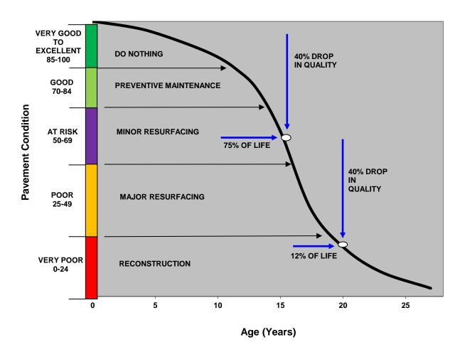
**Figure 3. Pavement Deterioration Curve**
