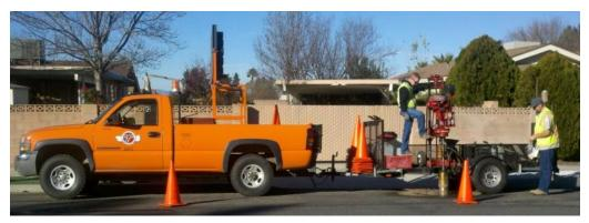
Figure 16. County's Coring Rig
