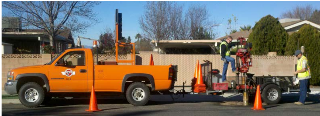
Figure 17. County's Coring Rig
