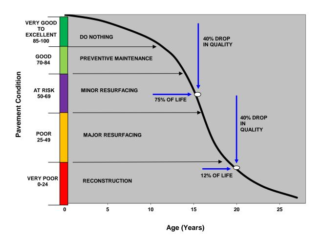
**Figure 9. Pavement Deterioration Curve**
