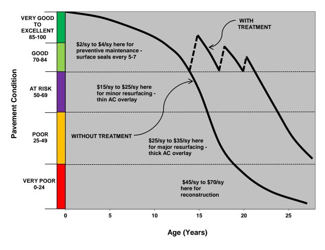
Figure 10. Pavement Deterioration Curve With and Without Treatment
