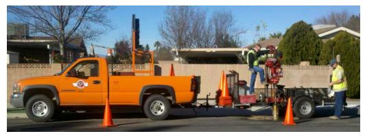
Figure 14. County's Coring Rig
