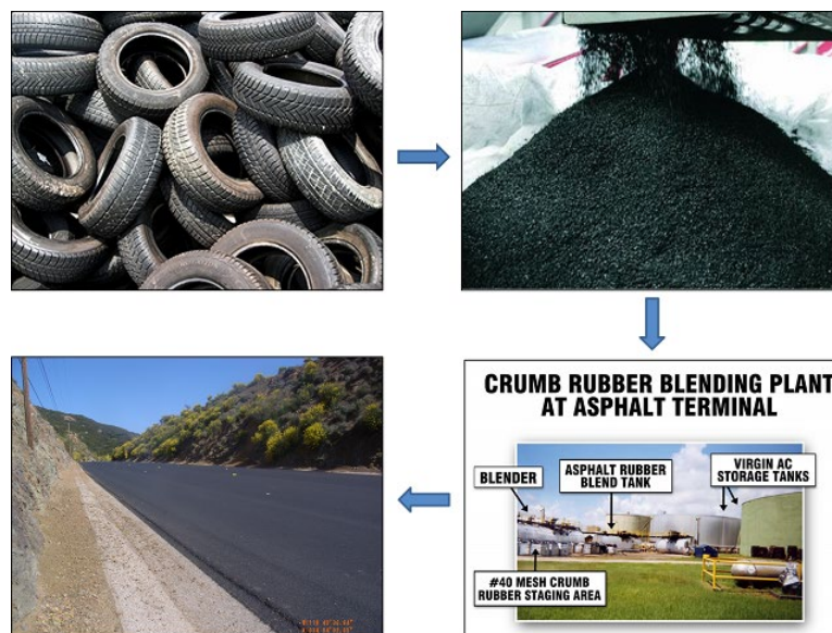
Figure 28. Rubberized Asphalt Concrete using Crumb Rubber
