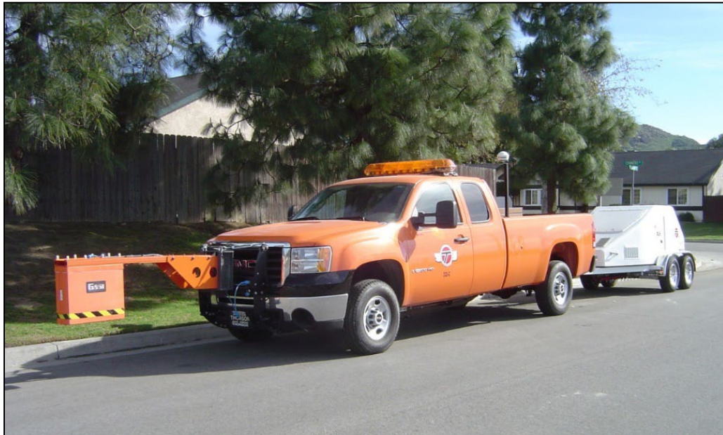
Figure 9. FWD and GPR Data Collection Equipment
