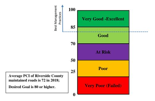
Figure 1. Relationship Between PCI and Pavement Condition
