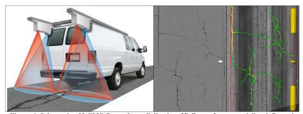
Figure 6. Schematic of LCMS Operation – Collection, 3D Range Image, and Crack Detection with Low and Medium Severity Cracks Identified
