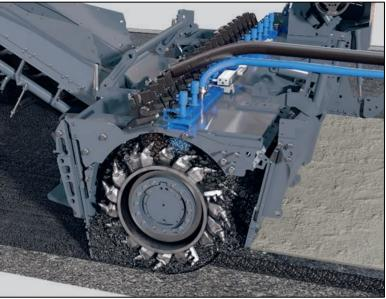
Figure 27. Cold In-Place Recycling (CIR)
