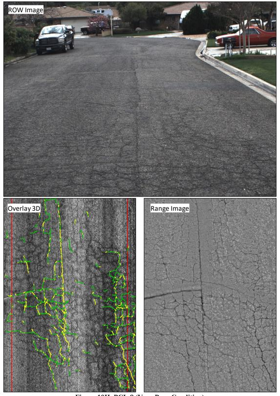
Figure 10H. PCI=8 (Very Poor Condition)
