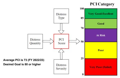
Figure 1. Relationship Between PCI and Pavement Condition
