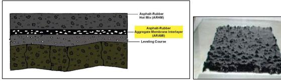
Figure 29. Asphalt Rubber Aggregate Membrane (ARAM)
