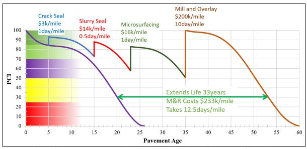
Figure 20. Treatment Zone Alternatives as a Function of Pavement Condition
